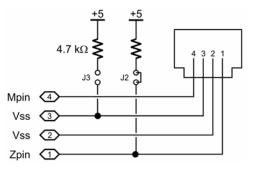
For 1-Wire I/O using a Blue Dot Receptor, configure the RJ-11 port as follows (J3 in, J2 out):
