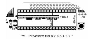
The BS1-IC can be programmed via the USB port or through a standard serial port when using the BS1 Serial Adapter (#27111, available separately) or the original parallel port programming cable (requires DOS editor that is no longer supported).
